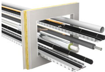
2. Mask the opening with crepe tape on all sides, keeping 20 mm distance to the edge. Coat the cables with FLAMMOTECT-A; alternatively apply fire protection wrap.
